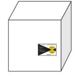
2. If the package is twice as long as it is wide, use two ShockWatch 2 Impact Indicators. Place a second indicator in the same position on the opposite side of the package.
