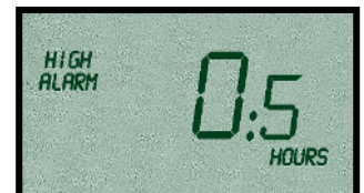
LCD displays the time above the specified high alarm setting for the current trip
